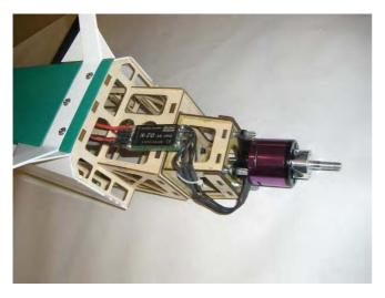
**step 4** Locate the ESC switch and fix it as per picture.
