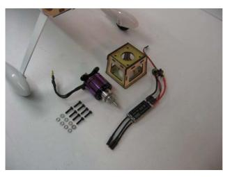
Locate the engine mount on the fuselage and glue it carefully with medium CA, than fix it using the four screws included in the hardware pack.
