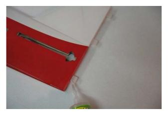
Drill in the rudder, 20mm from the bottom, the location for the tail wheel using a 2mm drill bit. Than locate the items included in the hardware pack, and assemble them as per picture.
