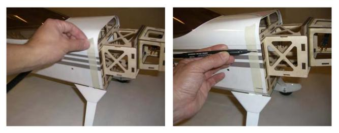
Slide the cowling onto the fuselage and install the spinner back plate. Position and hold the cowl so there is 3mm gap between the back plate and the cowl. Then apply another piece of masking tape on the same line of the one applied before.
