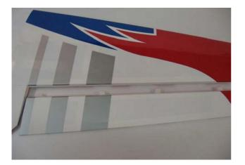
Carefully glue, with some drops of thin CA, each of the four hinges in the aileron.
