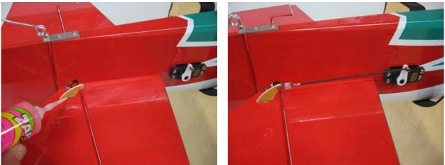
Section 7 – rudder servo & control horn installation
