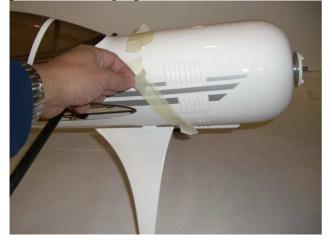
Drill the location for the four self-tapping screws using a 1.5mm drill bit.
