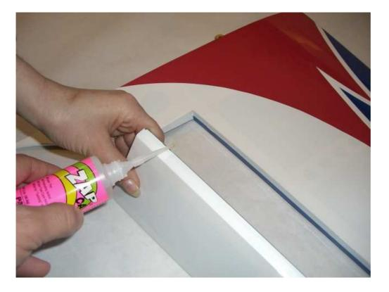
Locate the aileron and carefully glue, with some drops of thin CA, each of the four hinges into the wing panel.
