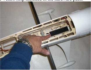
**step 2** Install the receiver, two extension 100mm for aileron servos and the battery pack as per the picture.
