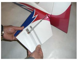
**step 4** Carefully glue the hinges in the stabilise with some drops of thin CA.
